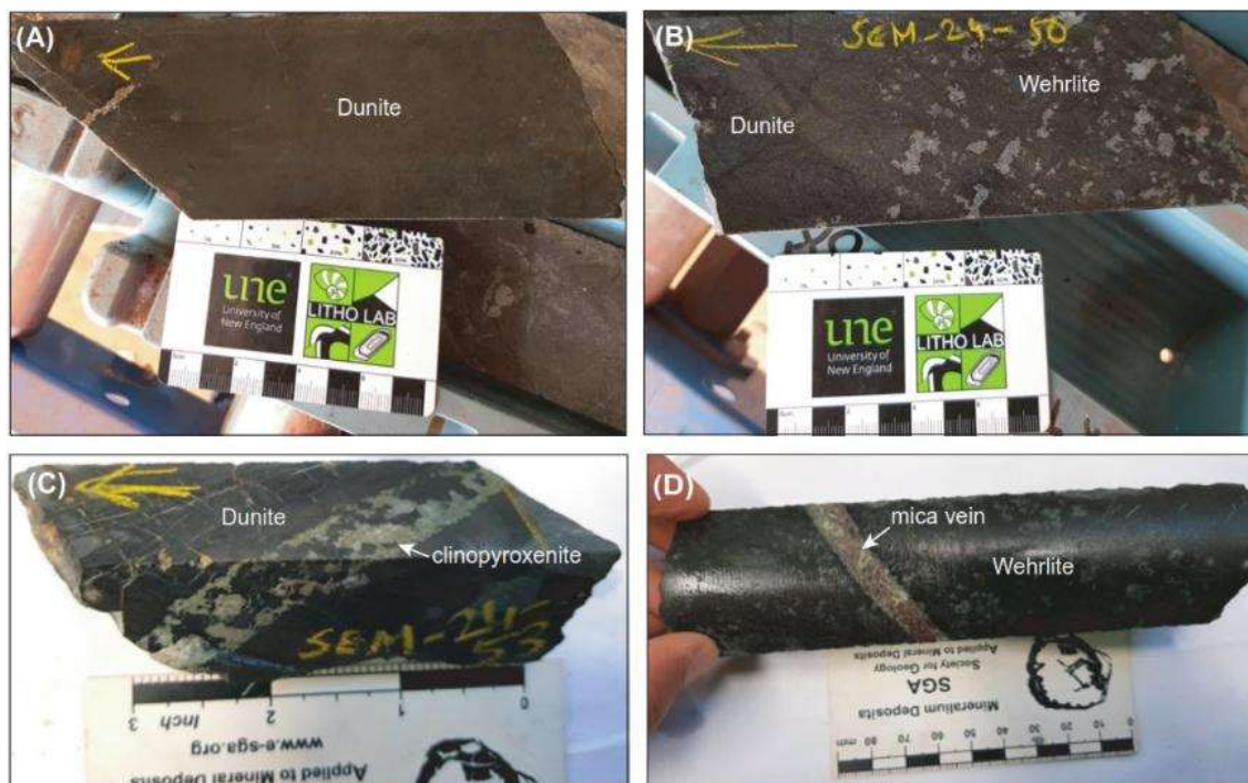
Figure 3. Hand specimen images of the primary ultramafic-mafic rocks sampled from diamond drill core SDD026 from the Tout Complex (A) Dunite (B) Dunite showing a gradational transition to Wehrlite (C) Dunite showing a distinct clinopyroxenite vein (1 cm wide) (D) Wehrlite showing mica vein (0.5 cm wide)
