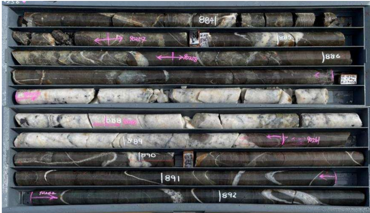
Figure 8. Foley Zone mineralised (wolframite) quartz vein within the Crescent Spur Sandstone in drill hole C2124A (completed in 2024), 2.47m @ 0.57% WO 3 from 887.0m
