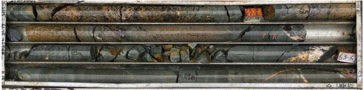
Figure 5. Drill core from drill hole C2115 (completed in 2117): 1.5m @ 0.83% Sn, 0.76% Cu & 10.4% Zn from 61.3m (Henry's Lode)
