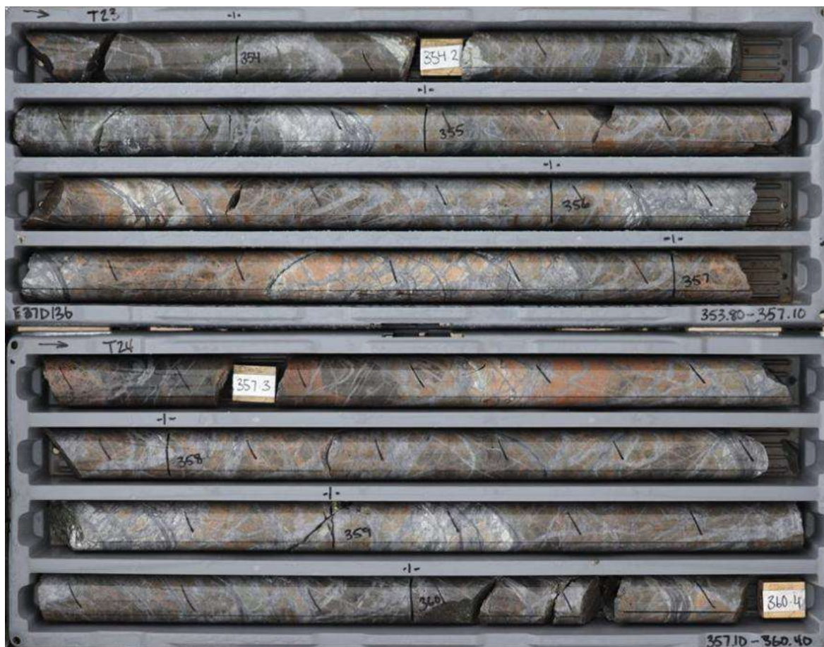
Figure 10: Intense quartz-bornite-chalcopryrite veining hosted in the Goonumbla Volcanics adjacent to the mineralising monzonite porphyry intrusion intersected in E37D136 from 353.8-360.4m.
