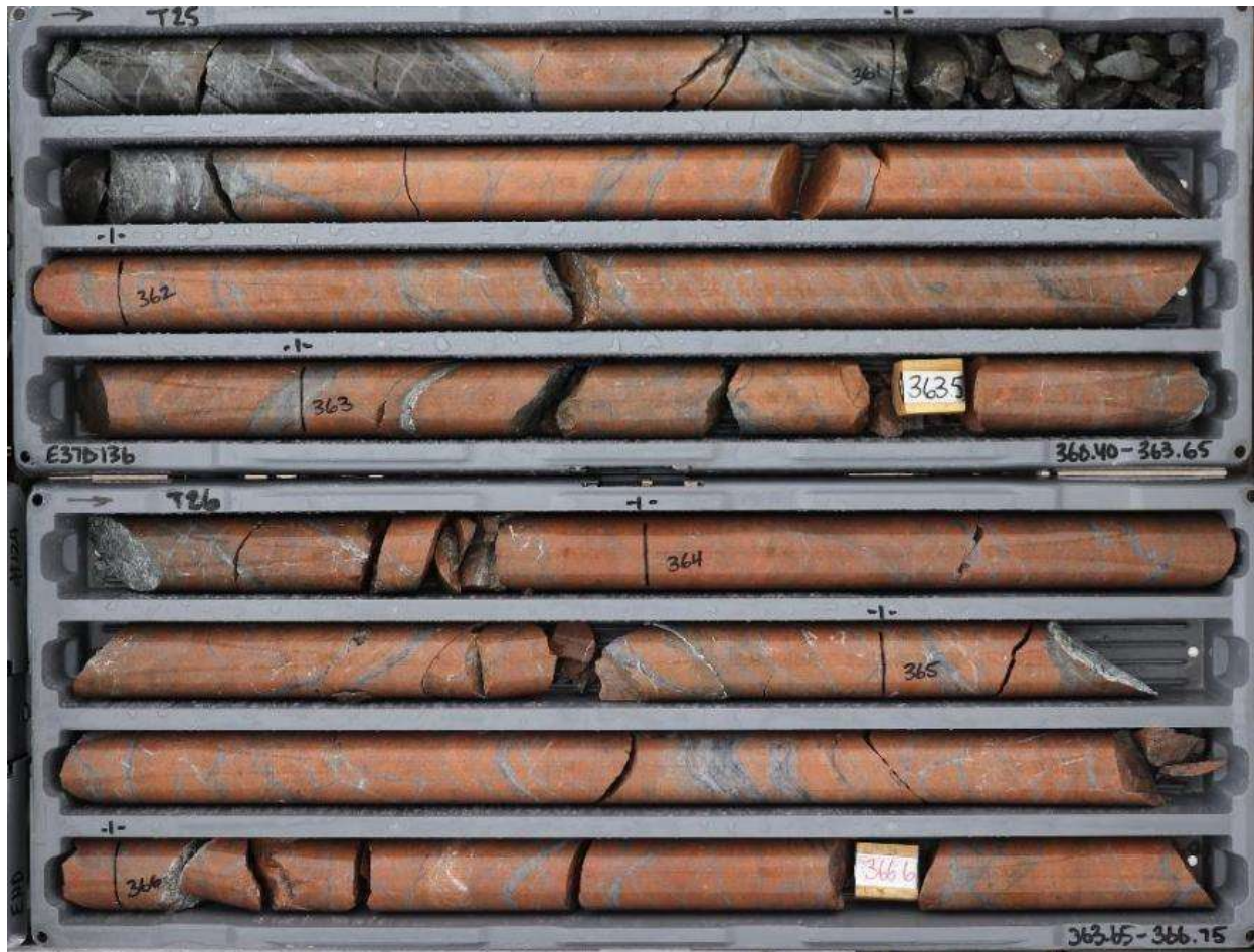
Figure 6: Mineralising monzonite porphyry intrusion from E37D136 from 360.4-366.75m
