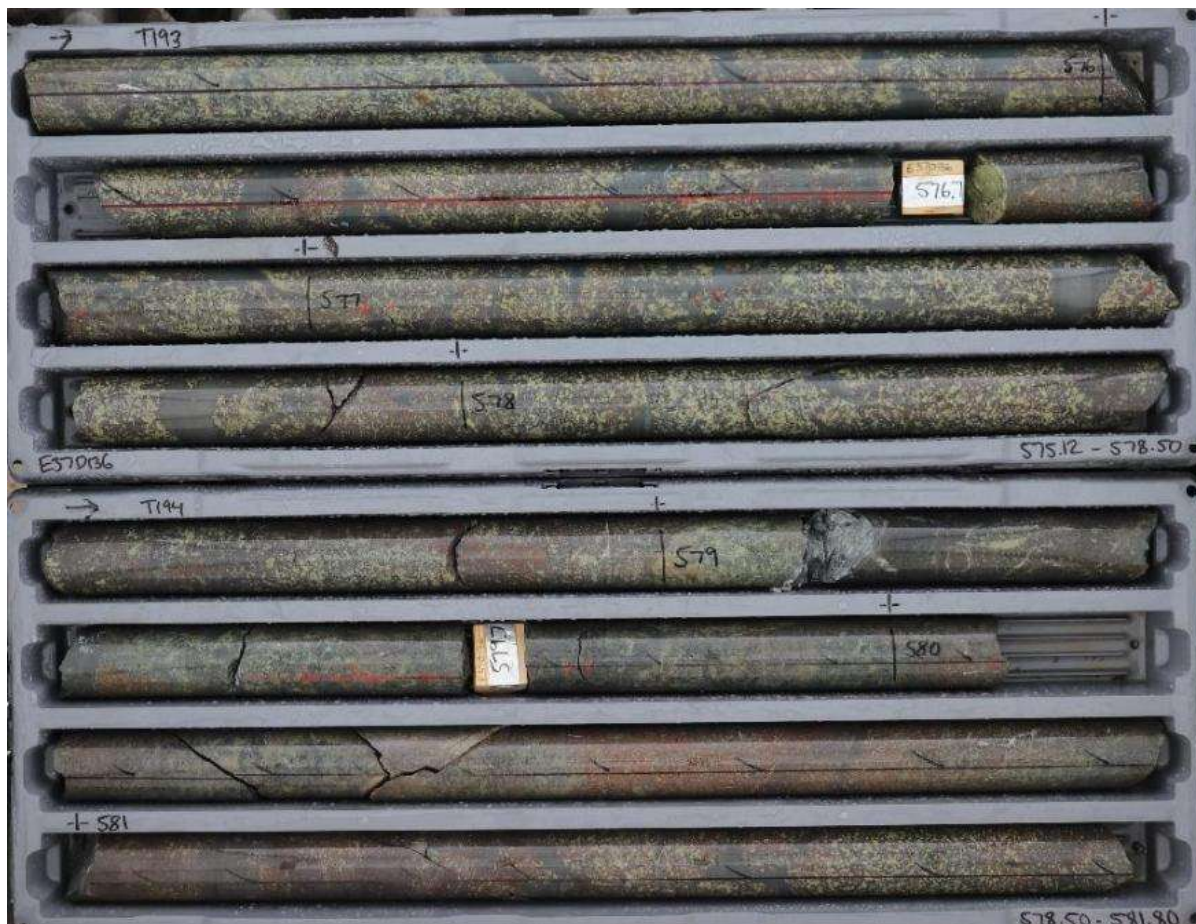
Figure 9: Epidote-chlorite-haematite propylitic altered peperitic andesite of the Goonumbla Volcanics intersected in E37D136 from 575.12-581.8m
