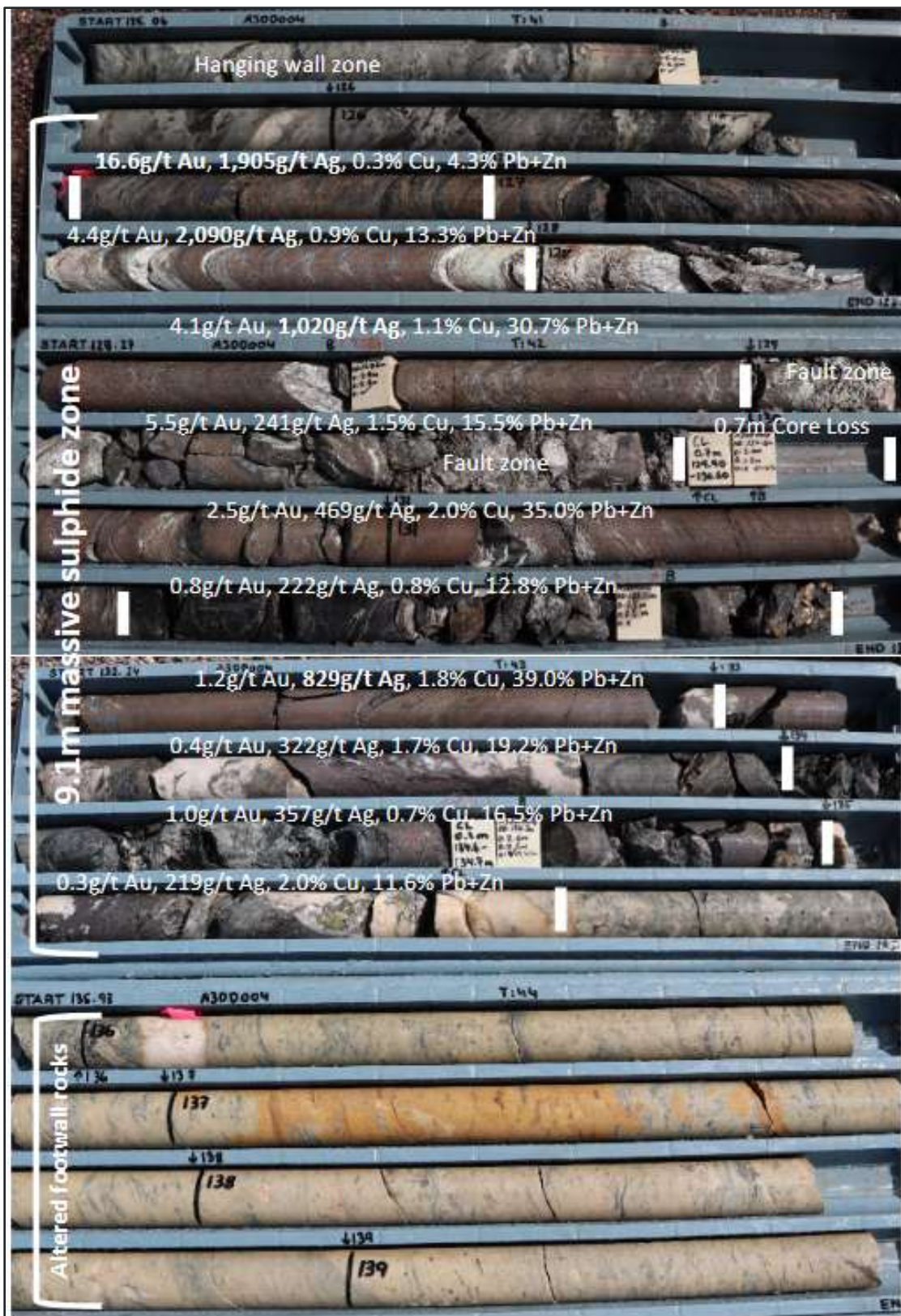
Figure 4 A3DD004 core with the Achilles Fault Zone, massive sulphides and intercept of 9.1m from 126.5m at 3.0g/t Au, 698g/t Ag, 19.4% Pb+Zn and 1.2% Cu, and altered pumice breccia in the footwall. AGC ASX announcement 13/11/2024
