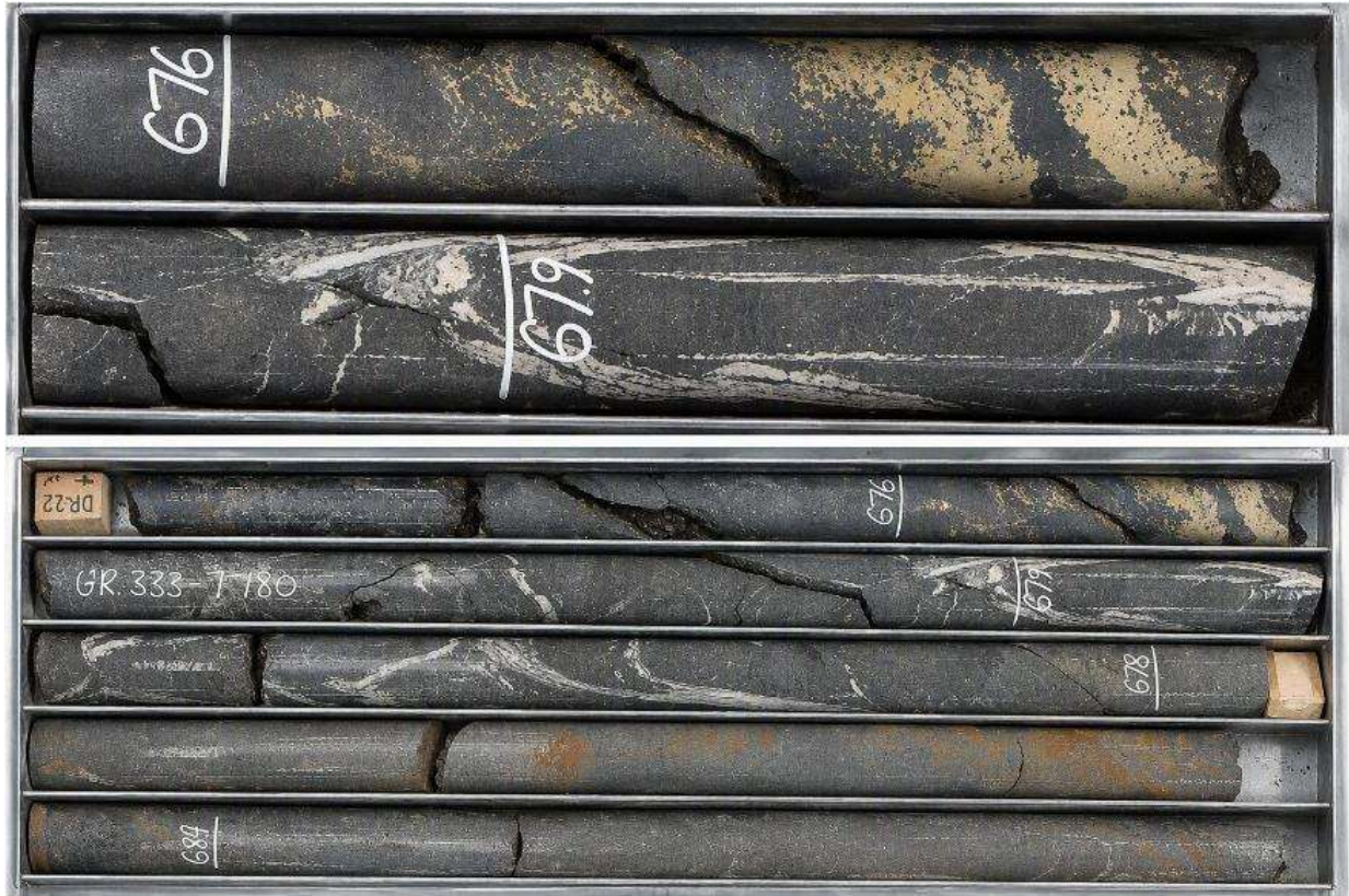
Figure 2 – Example of vein-hosted and disseminated sulphide mineralisation within a locally brecciated pyroxene porphyry dyke. Image of UR333 showing subsection of 16m @ 10.8g/t Au and 3.4% Cu.
