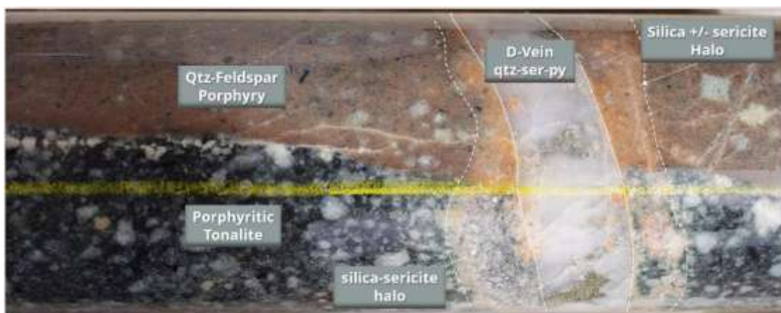
Figure 7. Porphyritic tonalite cut by a later quartz-feldspar porphyry and subsequently overprinted by a D-Vein.
