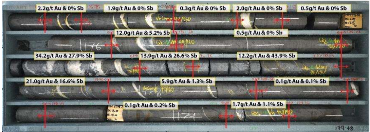
Figure 5. Drill core photos from BC418 (590 Vein) showing the nature of veining with individual assay grades of the samples. Composited interval graded 13.6g/t gold and 16.4% antimony over 2.22m (ETW 1.37m).
